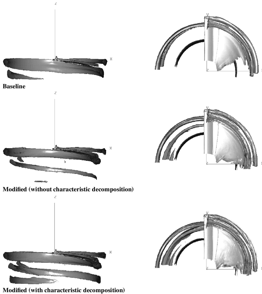
Fig. 4 Comparison between baseline TURNS code and modifications for the fine grid (isovorticity magnitude surface of value = 0.2).
